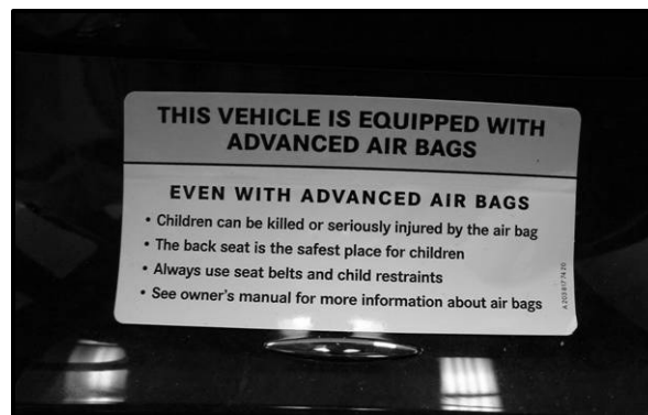
Additional label affixed to ash tray cover (Temporary label, removed after delivery)
